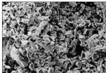
□ How diagenesis can affect permeability anisotropy. Pore-filling clay, such as this kaolinite, can destroy the permeability of this Bassien limestone.
