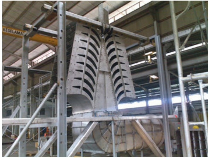
CONCEPT IVD separator inlet vane diffuser for a flare knockout drum assembled in a shop.
