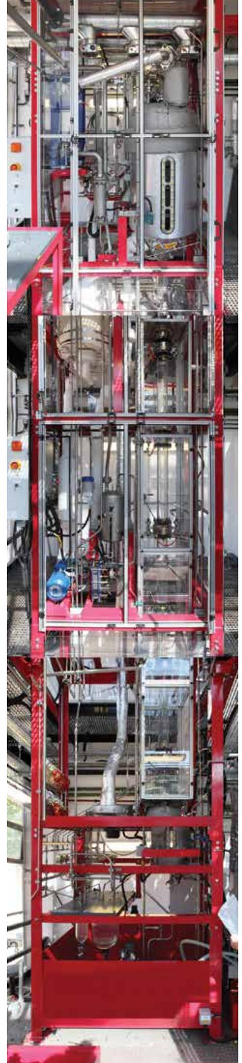
The PUREMEG system applies specialist experience and patented design features to optimize the extraction of large quantities of salt with reduced MEG losses, environmental impact, and down time.
