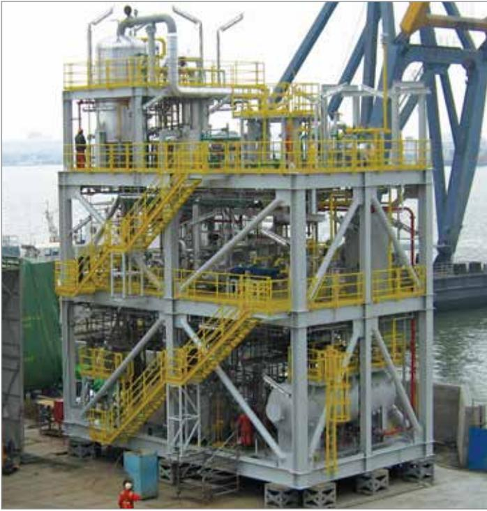
*Rich-MEG-flow 5-m<sup>3</sup>/h, 300-tonUK PUREMEG system module for offshore Brazil application.*
