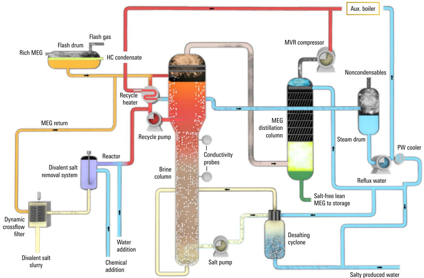
Typical PUREMEG system with mechanical vapor recompression.
