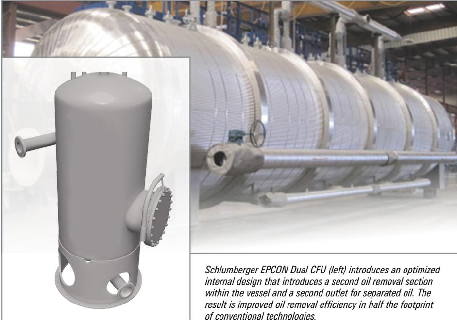
*Schlumberger EPCON Dual CFU (left) introduces an optimized internal design that introduces a second oil removal section within the vessel and a second outlet for separated oil. The result is improved oil removal efficiency in half the footprint of conventional technologies.*
