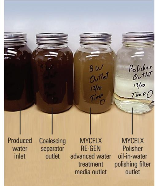
The inlet had contamination levels of 500–2,500 ppm of oil and grease with TSS of 2–100 ppm. After the suite of MYCELX technology was deployed, oil and grease at the final polisher outlet was below 10 ppm with a TSS below 10 ppm.
