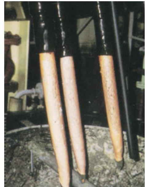
*Detailed shot of BFCC system electrodes installed in a marine (strainer-type) system.*
