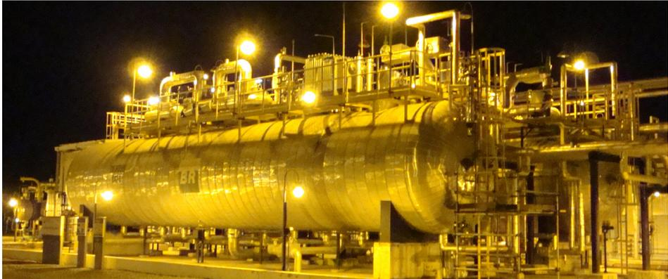
The Schlumberger BILECTRIC HF\* high-frequency AC desalter is the ideal solution for refinery desalting in which challenging crude slates, including low API and conductive crude oils, are present.
