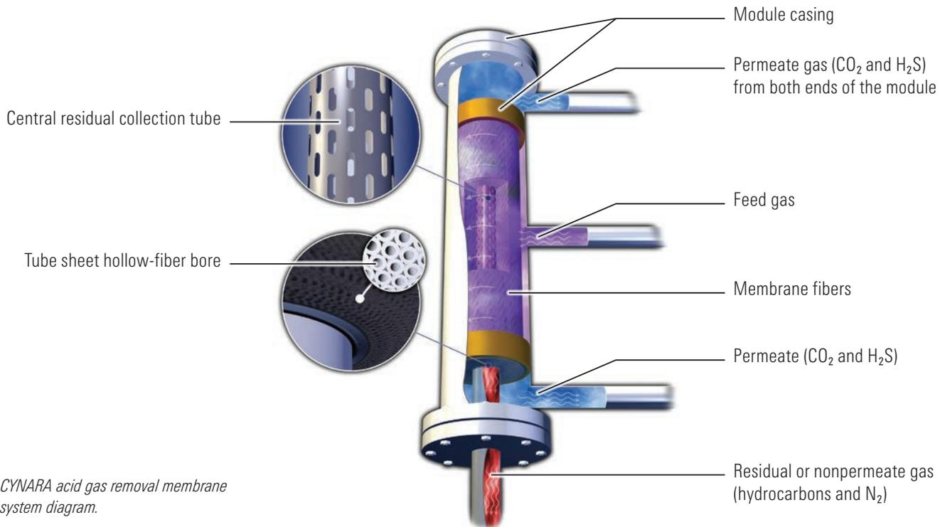
*CYNARA acid gas removal membrane system diagram.*
