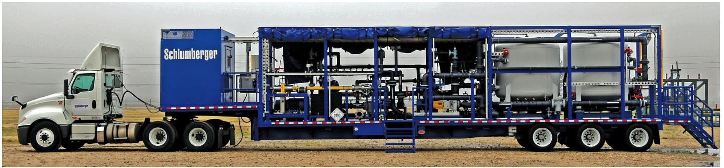
*The DT trailer treats produced and flowback water, delivering up to 17,000 bbl/d of frac-grade water.*
