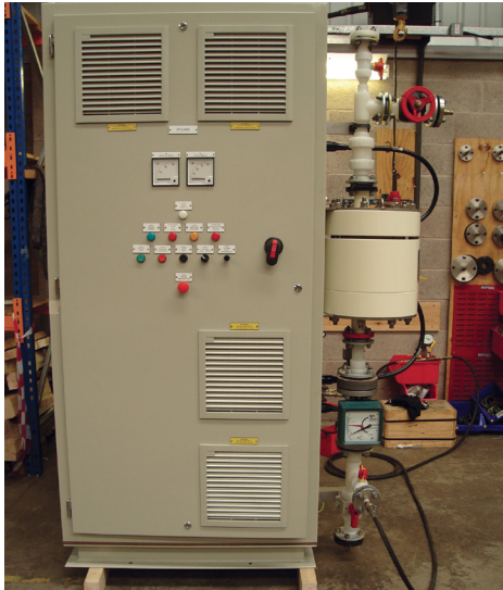
Standard SEA-CELL electrochlorinator with integrated power and control panel.
