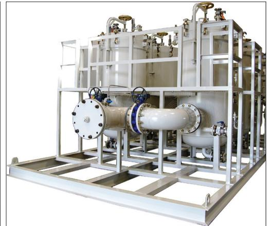
Skid-mounted MYCELX Polisher filter unit ready for delivery.
