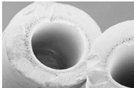
Each membrane module consists of a pressure vessel that houses a number of membrane bundles, with each bundle comprising hundreds of hollow membrane fibers. Feedwater flows from the outside of the membrane to the inside before exiting the vessel. The module is installed in a vertical position.
