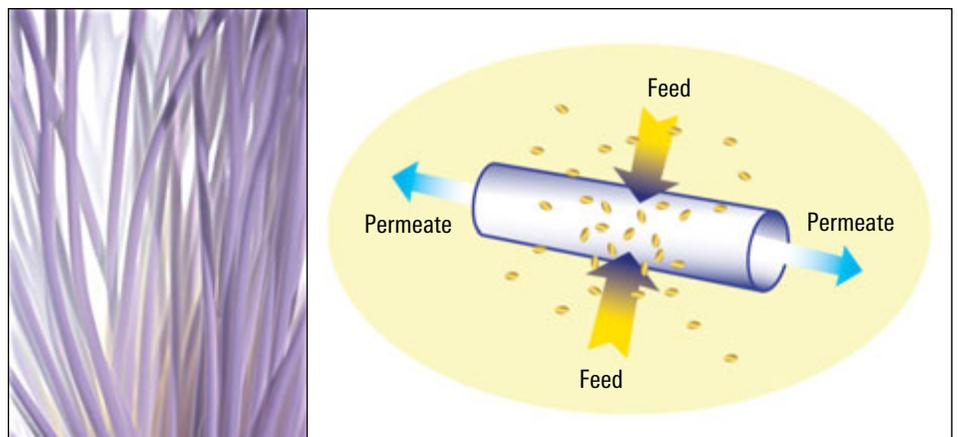
Close view of a UF membrane fiber.
