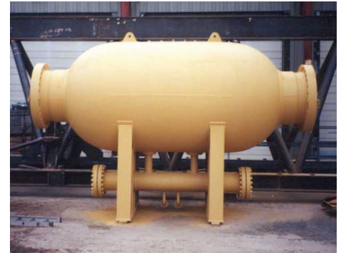
PORTA-TEST WHIRLYSCRUB I Model C separator, capable of handling 3.6 Bcf/d.
