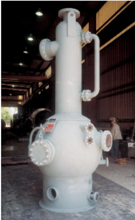
PORTA-TEST WHIRLYSCRUB V gas scrubber with oversized liquid chamber.
