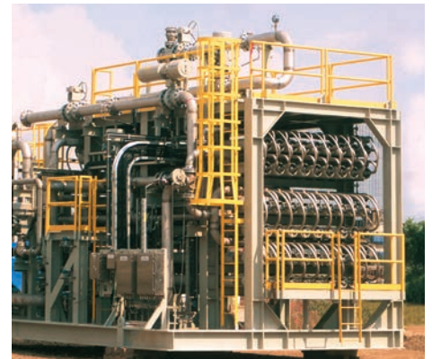
One of seven sulfate removal modules capable of producing 50,000 bbl/d [330 m 3 /h] of low-sulfate seawater for Kizomba A Field, West Africa.
