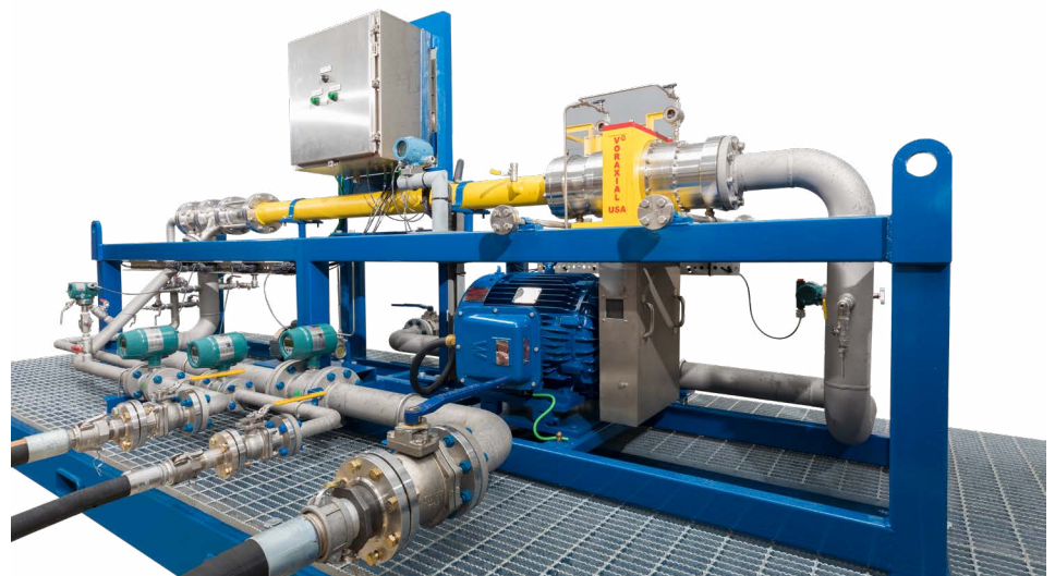
The Voraxial impeller-induced cyclonic separator uses a unique no-shear impeller to induce radial and axial flow for three-way separation of water, oil, and solids.
