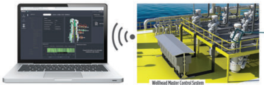
Fig. 2. The all-electric surface actuator enables remote valve operation and health monitoring, saving costs by reducing visits to offshore platforms and remote locations.
