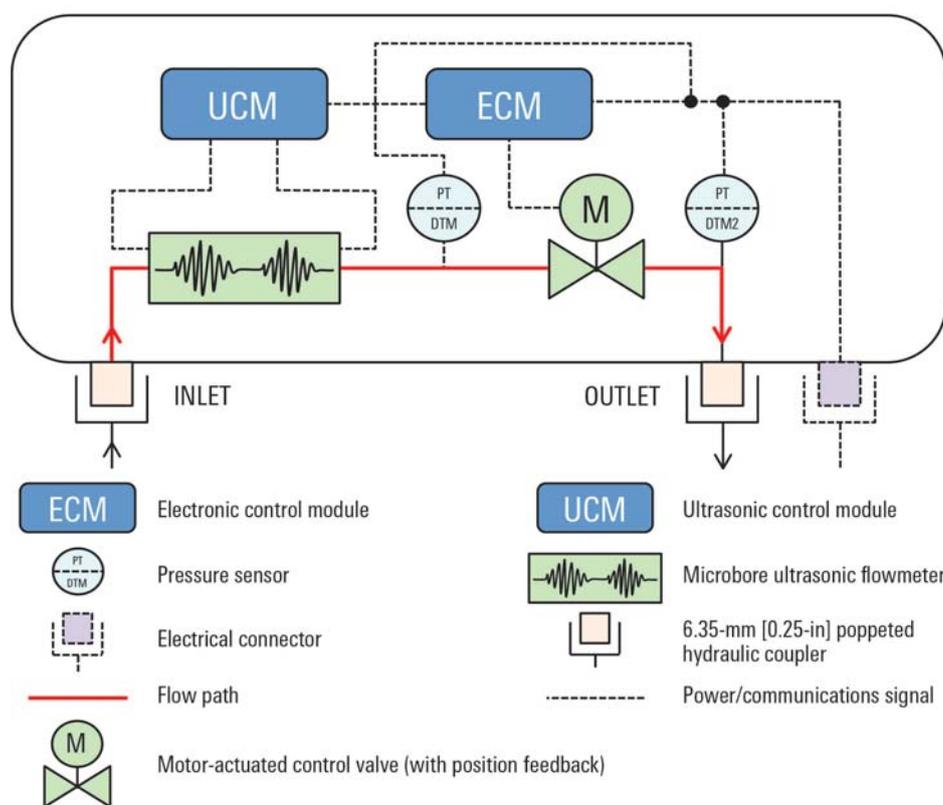
Figure 3: PULSE CIMV system architecture (Image: Schlumberger)
