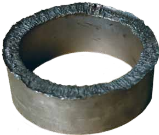
The high-quality cut of this 5 \frac{1}{2} -in 26-lbm/ft 25% chrome tailpipe was obtained with the 4.15-in PowerCutter tool, which can pass through a 4.25-in subsea safety valve.
