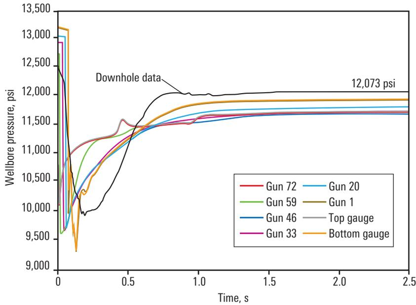
Downhole gauges confirmed that the measured peak dynamic underbalance correlated with the pressure simulated prejob in SPAN Rock analysis. The rapid drop in pressure removed skin damage, creating cleaner perforating and improving the productivity index.
