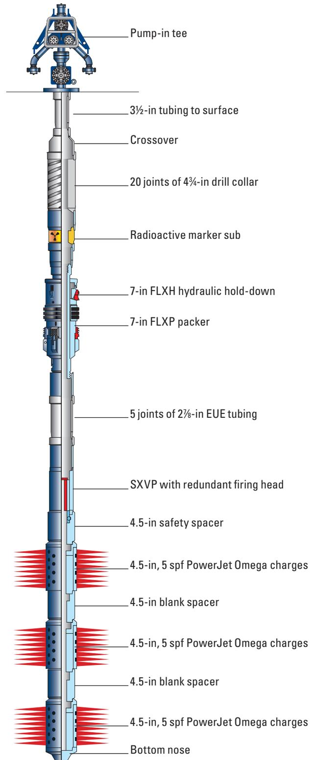
*Tubing-conveyed perforating string configuration with PowerJet Omega charges.*
