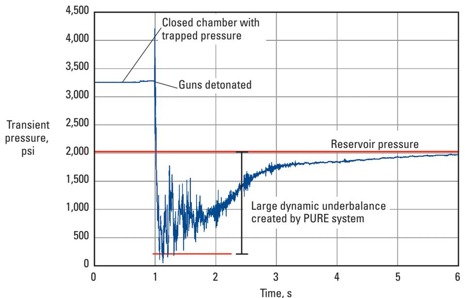
The PURE system delivered clean perforations, as demonstrated by analyzing the pressure transient data acquired at a 1-ms rate by the fast gauge.
