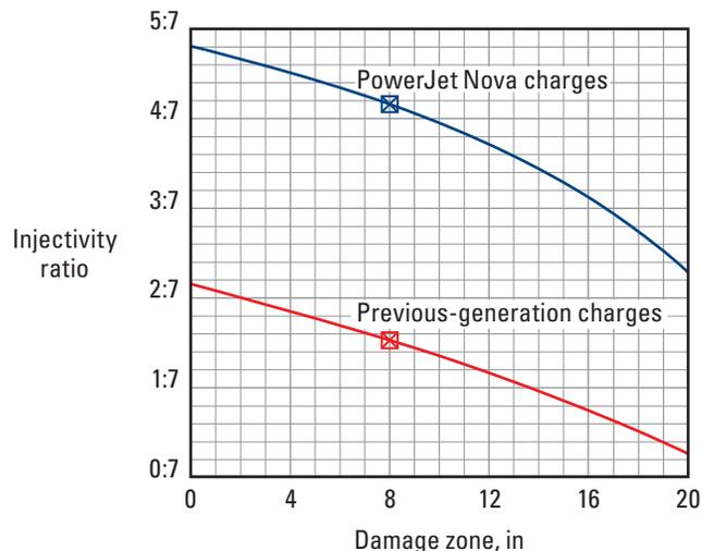
A plot derived from SPAN Rock software shows that using PowerJet Nova charges would provide the best injectivity performance for the job.
