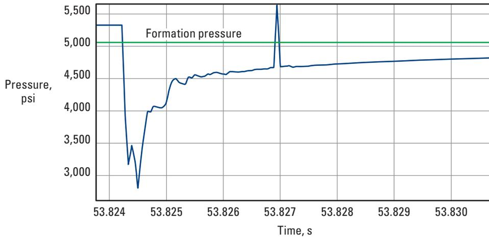
A downhole gauge captured the 2,500-psi [17.2-MPa] underbalance created by the PURE system. This dynamic underbalance removed perforation debris from tunnels immediately after guns fired.
