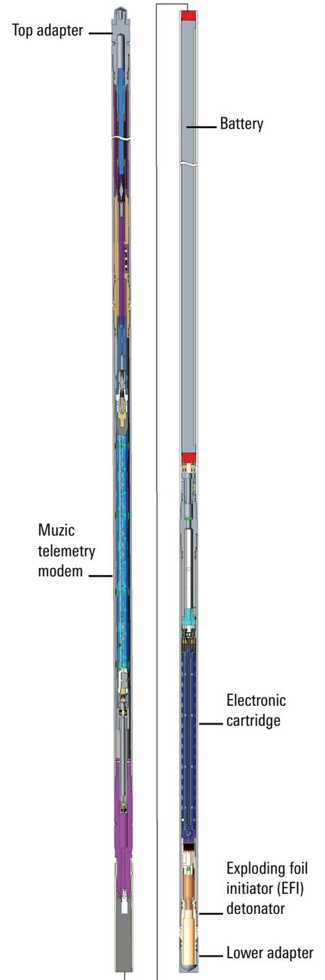
*eFire-TCP tubing-conveyed perforating electronic firing head enabled by Muzic wireless telemetry.*
