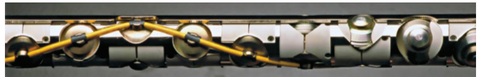
2 1/8-in PowerSpiral Nova spiral-phased capsule perforating system, 6 spf, 45° pendulum phasing.
