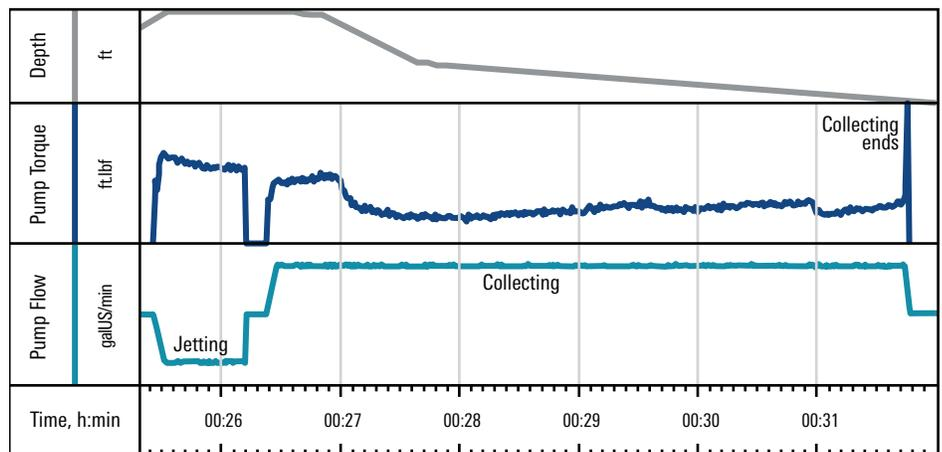
Real-time monitoring of ReSOLVE service’s debris removal tool shows the precise control applied to the downhole debris collection.
