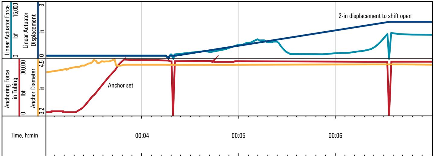
Real-time monitoring verified the progress of the linear actuator tool in successfully shifting the valve by 2 in with a maximum force of 15,000 lbf.
