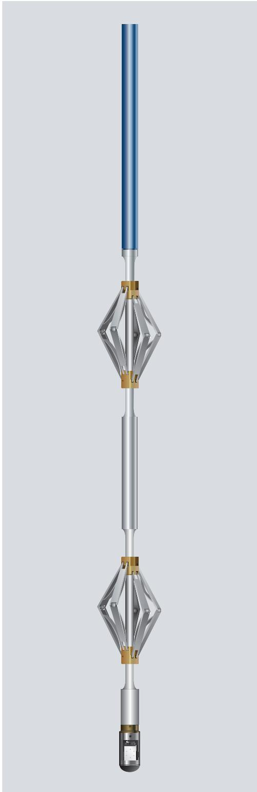
The UCI\* Ultrasonic Casing Imager is an evolution of the USI\* UltraSonic Imager. The UCI tool provides all the answers required to locate, identify, and quantify casing damage or corrosion. The design is specifically engineered for high-azimuthal-resolution images and detailed examination of both the inner and outer surfaces of casing ranging from 4½ to 13¾ in. [11.43 to 33.97 cm] resulting in improved echo detection.
