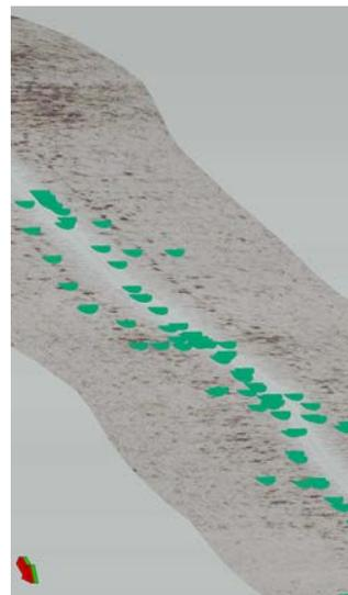
Migrated image plus events from 3D far-field sonic imaging showing the presence of fractures deep into the formation.
