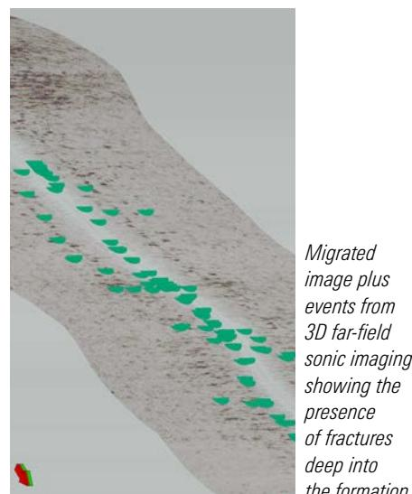
Migrated image plus events from 3D far-field sonic imaging showing the presence of fractures deep into the formation.
