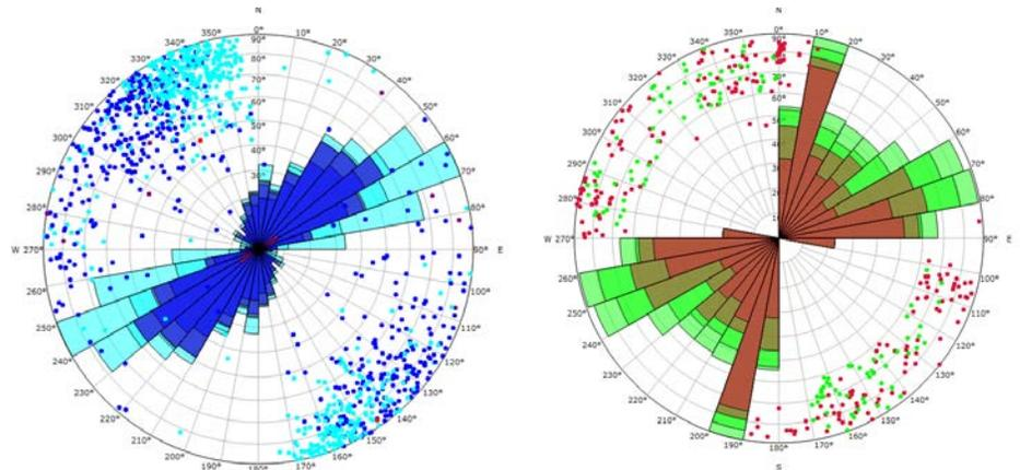
Rose plot of natural fractures from through-the-bit logging (left) and fracture-related events from 3D far-field sonic imaging using slim dipole logging conveyance (right).
