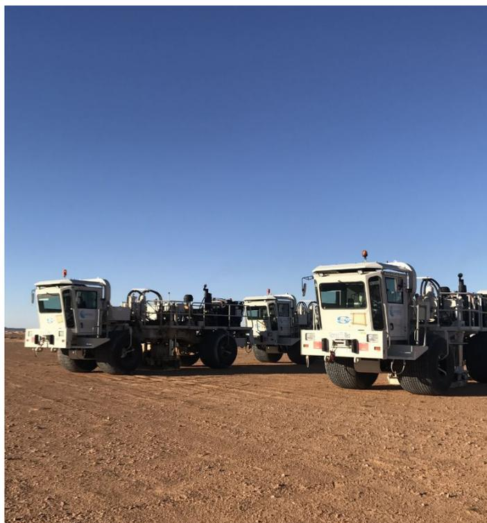
Figure 2. 65,000-lbm vibroseis fleet used for the acquisition.
