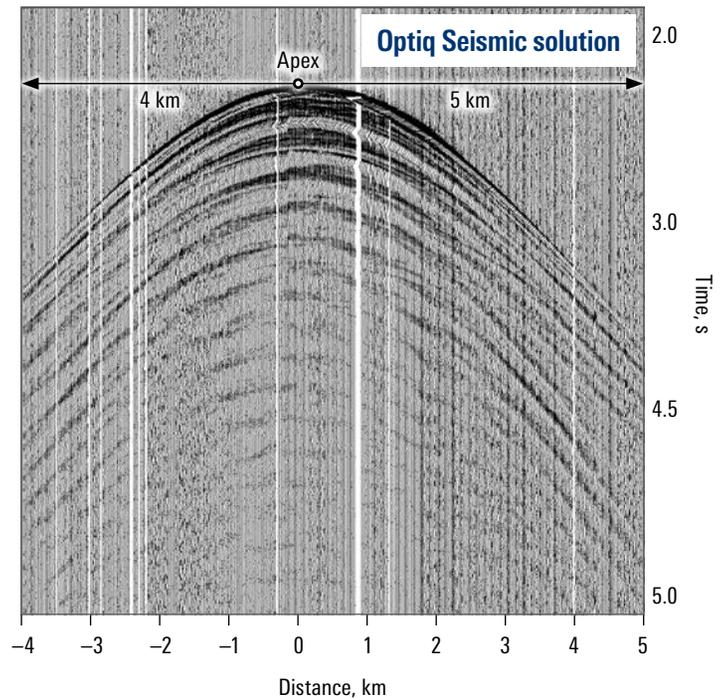
The Optiq Seismic solution walkaway survey receiver gather of field raw shots shows good signal-to-noise ratio. The image shows an asymmetric line with 4-km offset to the left of the apex and 5 km to the right, with 360 shots at 25 m with gaps. The signature changes are due to pressure drop.
