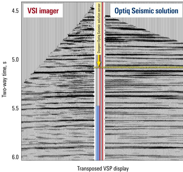
The transposed zero-offset VSP data from the VSI imager and Optiq Seismic solution shows upgoing waves deconvolved to zero-phase over 4–80 Hz. In this type of display, the most accurate data is in the center, where it is easier to correlate different upgoing datasets.
