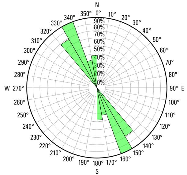
Figure 3. Fast shear azimuth for dipole anisotropy >5% indicates for this example the maximum horizontal stress direction.
