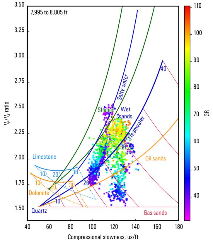
Figure 4. This crossplot illustrates changes in  $V_p/V_s$  for the respective lithologies (color is a function of shale content) as a function of the compressional slowness. The crossplot is also often used to discriminate light hydrocarbon-bearing intervals from water-bearing intervals.
