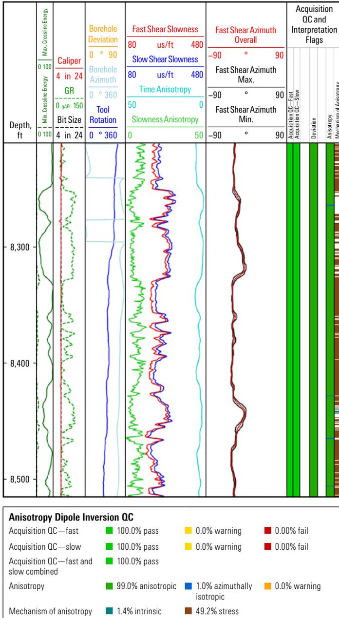
Figure 2. The dipole anisotropy results for the same logged interval showing a consistent shear polarization direction with valid fast and slow shear slownesses. The summary of the QC for the dipole anisotropy indicates that most of the section shows stress-induced anisotropy, which was also confirmed using the dispersion analysis.
