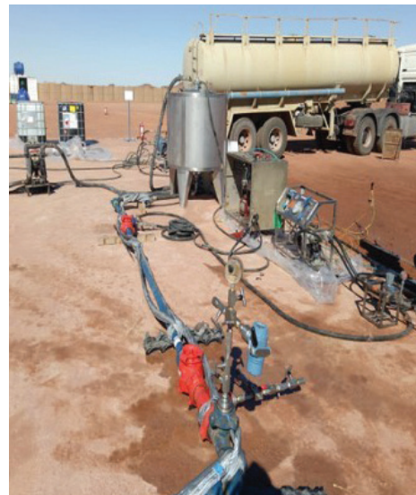
High-quality resin was integrated into a mobile package consisting of a customized set of surface equipment, chemical pumps, and mixing tanks.
