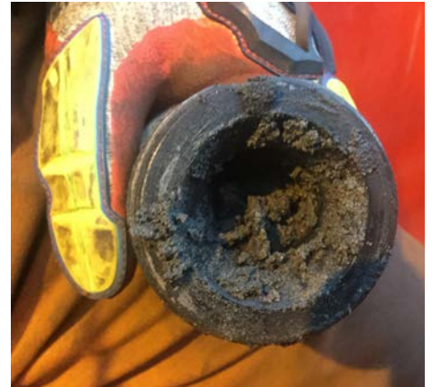
Perforation cleanout chamber returned to the surface following a P3* postperforating treatment run.
