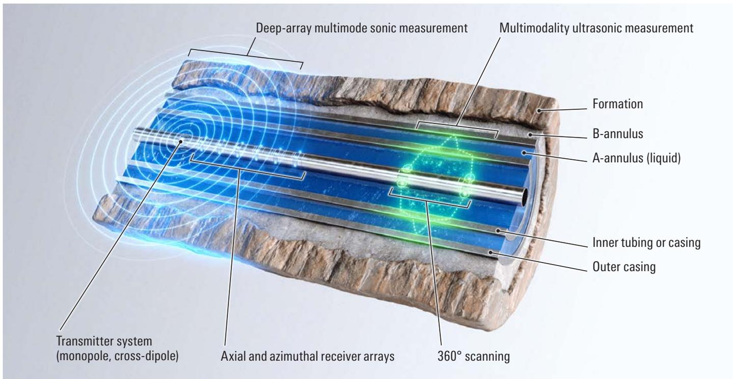
Dual-string P&A barrier evaluation enables A- and B-annuli barrier logging without removing the inner pipe.
