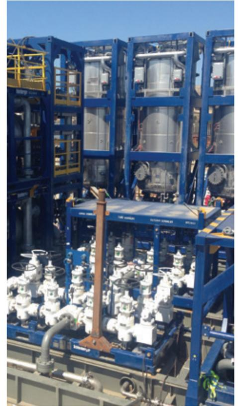
*The package is pictured with the choke manifold, surge tanks, separator, and steam exchangers.*
