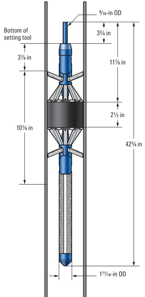
4½-in or 5-in PosiSet mechanical plugback tool with 1<sup>11</sup>/<sub>16</sub>-in OD.
