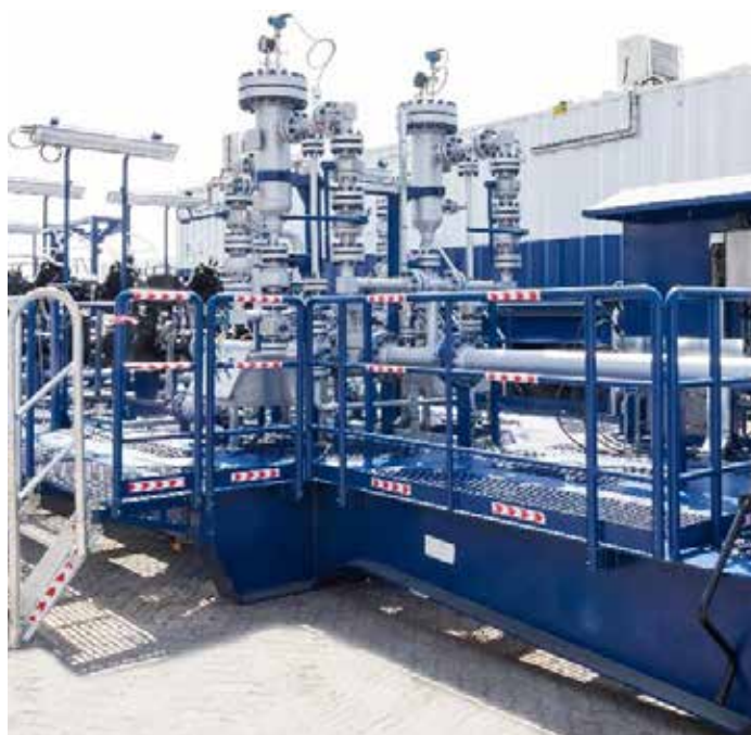
Example of a trailer-mounted underbalanced drilling package.
