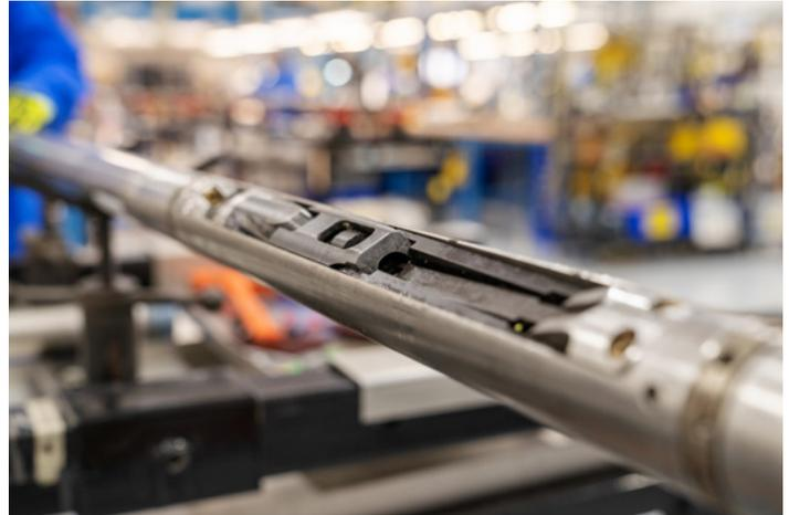
*Anchor tool of ReSOLVE iX service slot cutter.*
