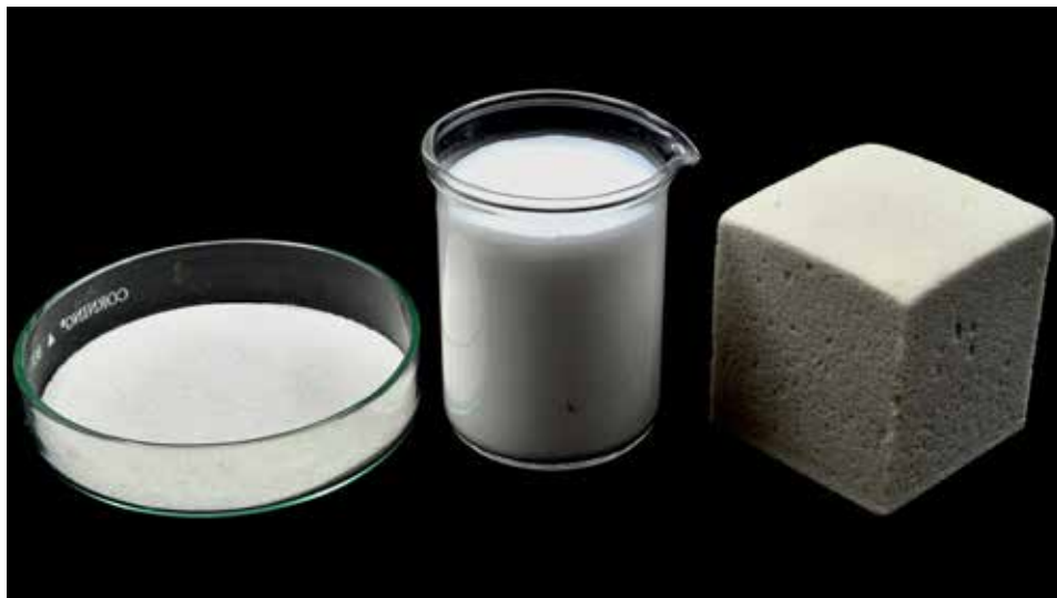
Column of consolidated sand (right) formed by combining fluids from the water-based sand consolidation system (center) and unconsolidated sand (left).
