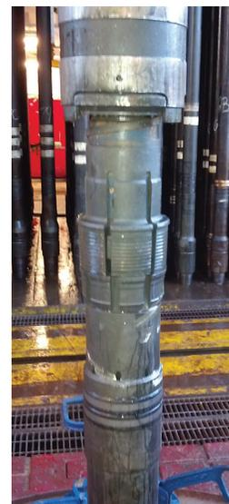
*The multifunction 10K ASST set the gravel-pack packer and eliminated unwanted swabbing effects as well as a separate trip for filtercake removal.*
