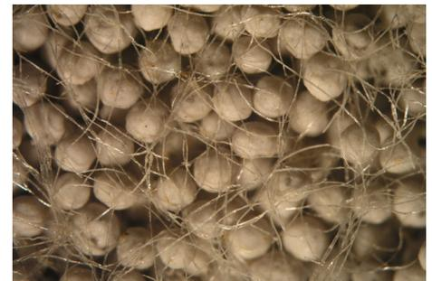
Interconnected network of fibers providing stability in the sample (magnified view).
