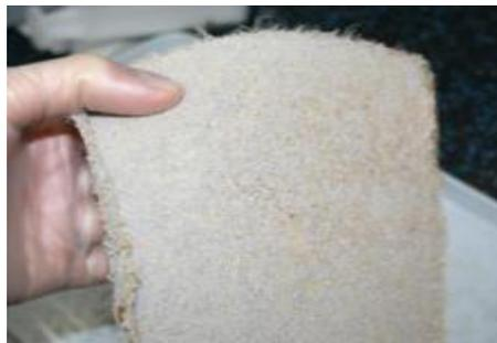
Sample of 20/40 ceramic proppant with 1.2% BWOP activated FiberPAC technology.
