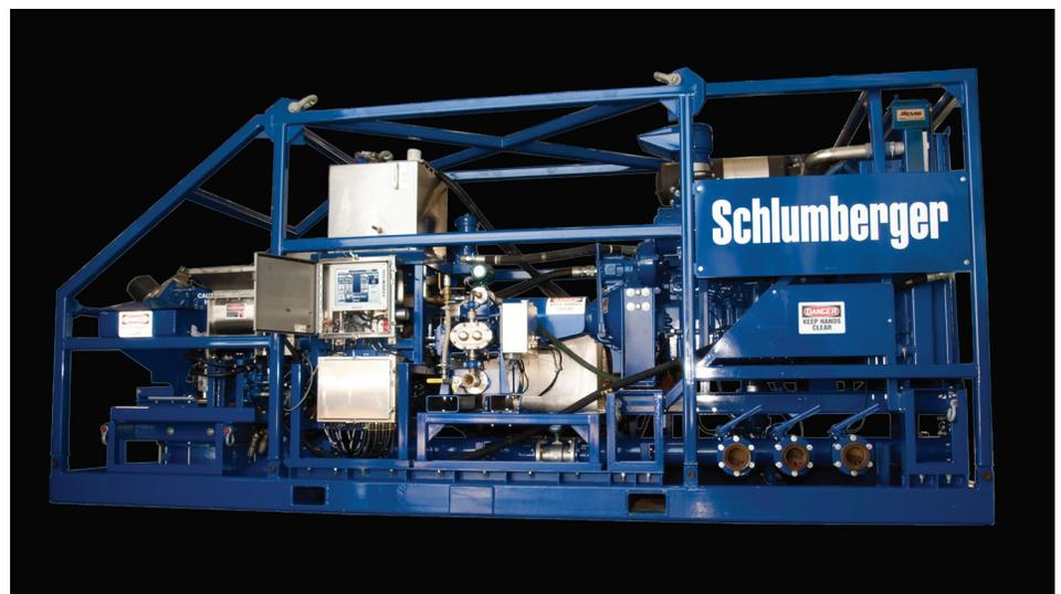
*Hornet skid-mounted blender for use with slurried gravel-pack fluids.*
