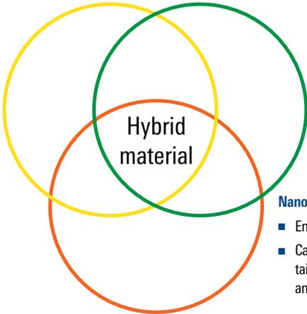
*The Nanoglue bond is made of a nanostructured, silica-based inorganic component blended with an organic polymer precursor. Interpenetrating polymeric networks link the organic and inorganic components on a nanometer scale. After it is cured, the inorganic and organic components form a hybrid material with a strong attraction to a sand surface and enhanced physical and chemical properties.*
