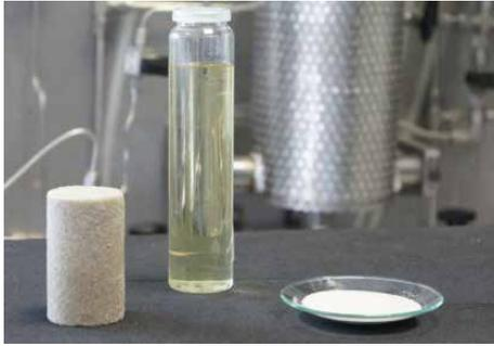
*The column of consolidated sand (left) was formed by combining Nanoglue bond (center) and sand (right).*
