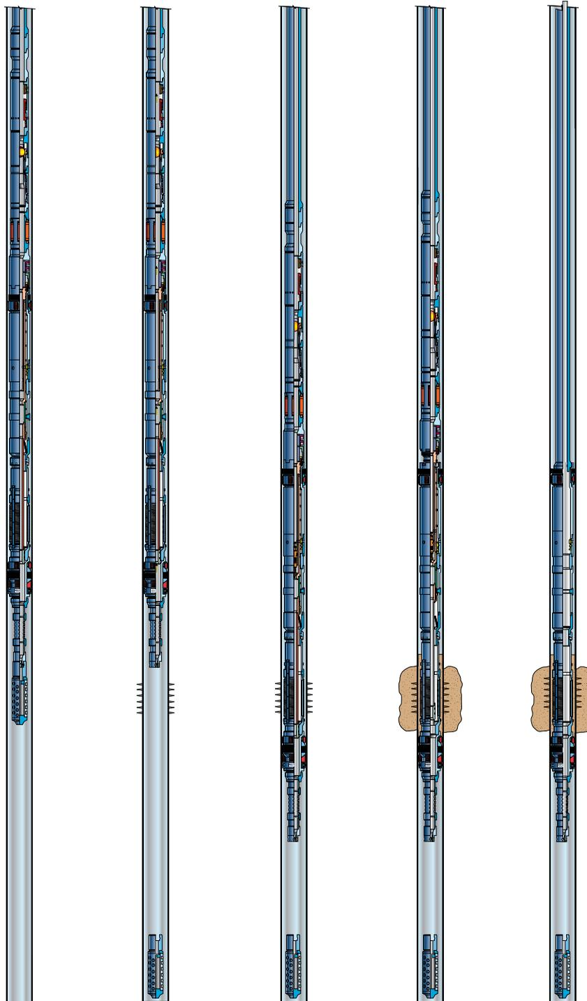
Run bottomhole assembly to perforation depth
