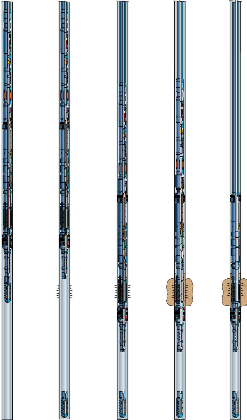
Run bottomhole assembly to perforation depth
