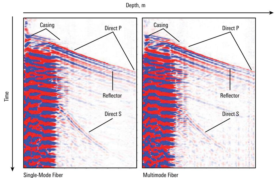
The hDVS DAS system acquired VSPs with a strong reflector and P and S arrivals using either the single-mode and multimode optical fibers, at distances of more than 5 km and less than 1 km, respectively, from the system’s interrogator.
