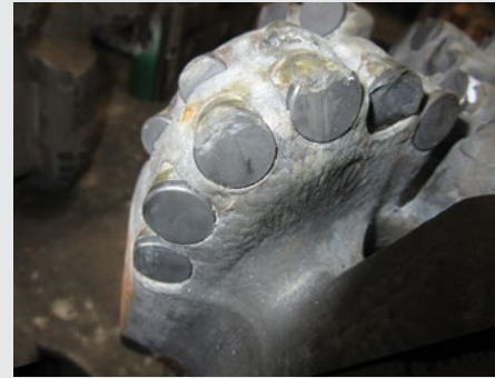
The dull condition of previous-generation PDC technology showed considerable damage in this application.
