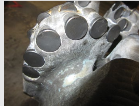
The cutters using FireStorm technology demonstrated better resistance to wear and impact.
