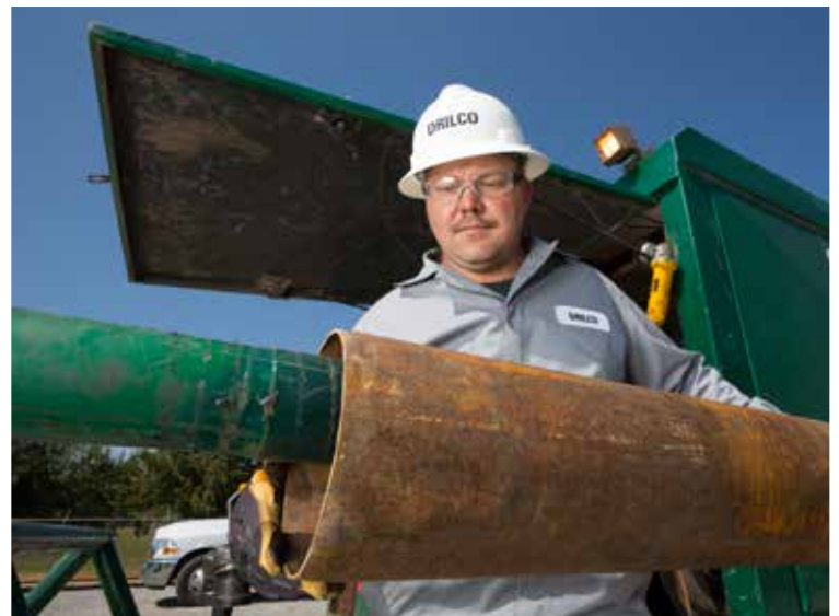
DRILCO personnel preheat tubulars prior to the hardbanding process to ensure the correct and consistent application of hardbanding material.
