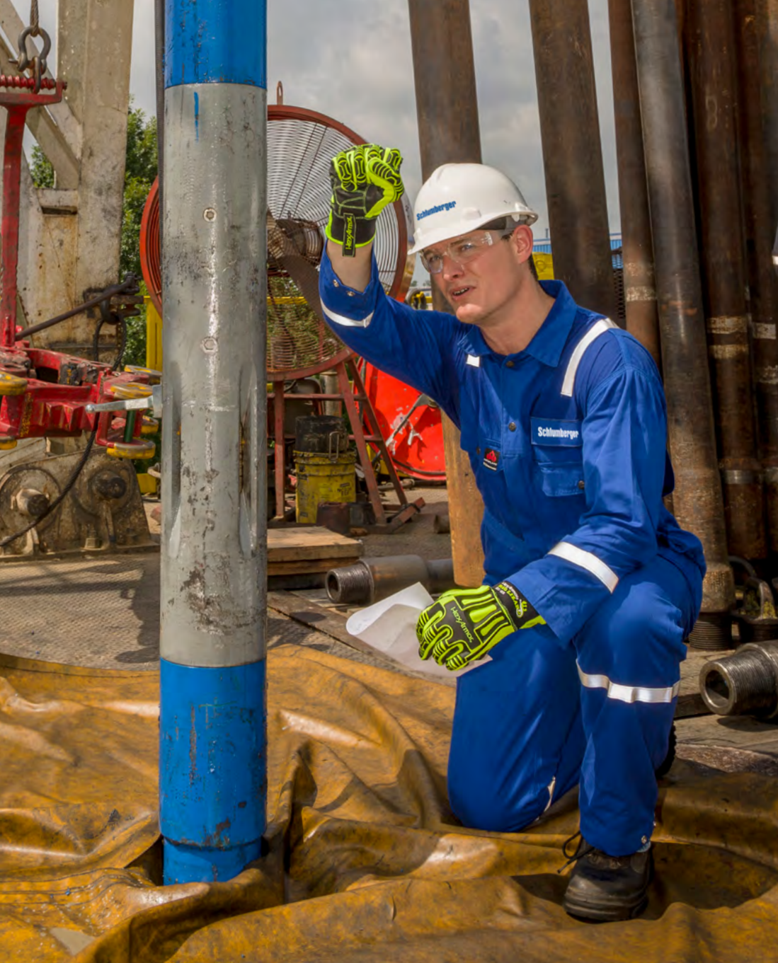
The Rhino XC reamer can be tested at the surface to check settings prior to being run in the hole.
