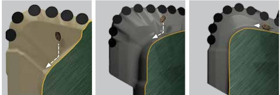
*The next-generation Spear bit features an improved bullet-shaped profile (left). The steeper gradient provides more effective cuttings evacuation than the first-generation Spear (middle) and a standard matrix PDC bit profile (right).*
