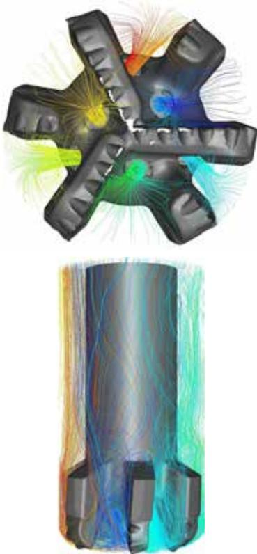
*The next-generation Spear bit's advanced hydraulics maximizes cutting structure cleaning and junk slot flow.*
