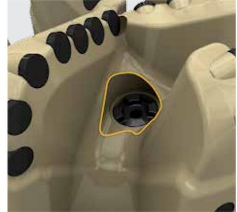
*A shale evacuation channel is formed on the bit body near the nozzle bores providing an unobstructed flow path for cuttings evacuation, which greatly reduces blade packing and nozzle plugging.*
